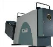
Mechelle 5000- Spectrograph Designed to provide simultaneous recording from 200-975 nm in one acquisition.
